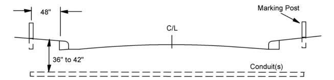
Note: For Multiple Conduits, a 12" Separation is Required.
