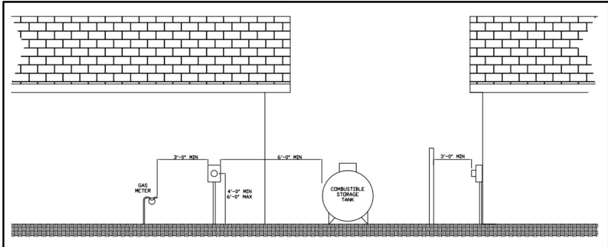
Figure 12. – Customer Peak Shaving DER Minimum SCADA Wiring
