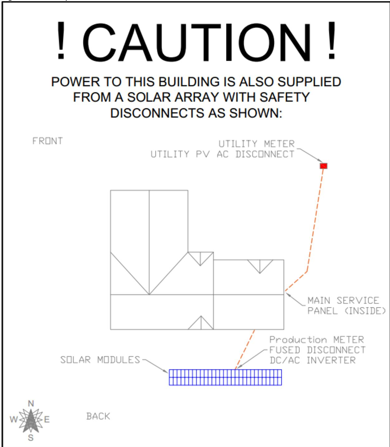
Figure 11. Metering Profile Elevation Drawing
