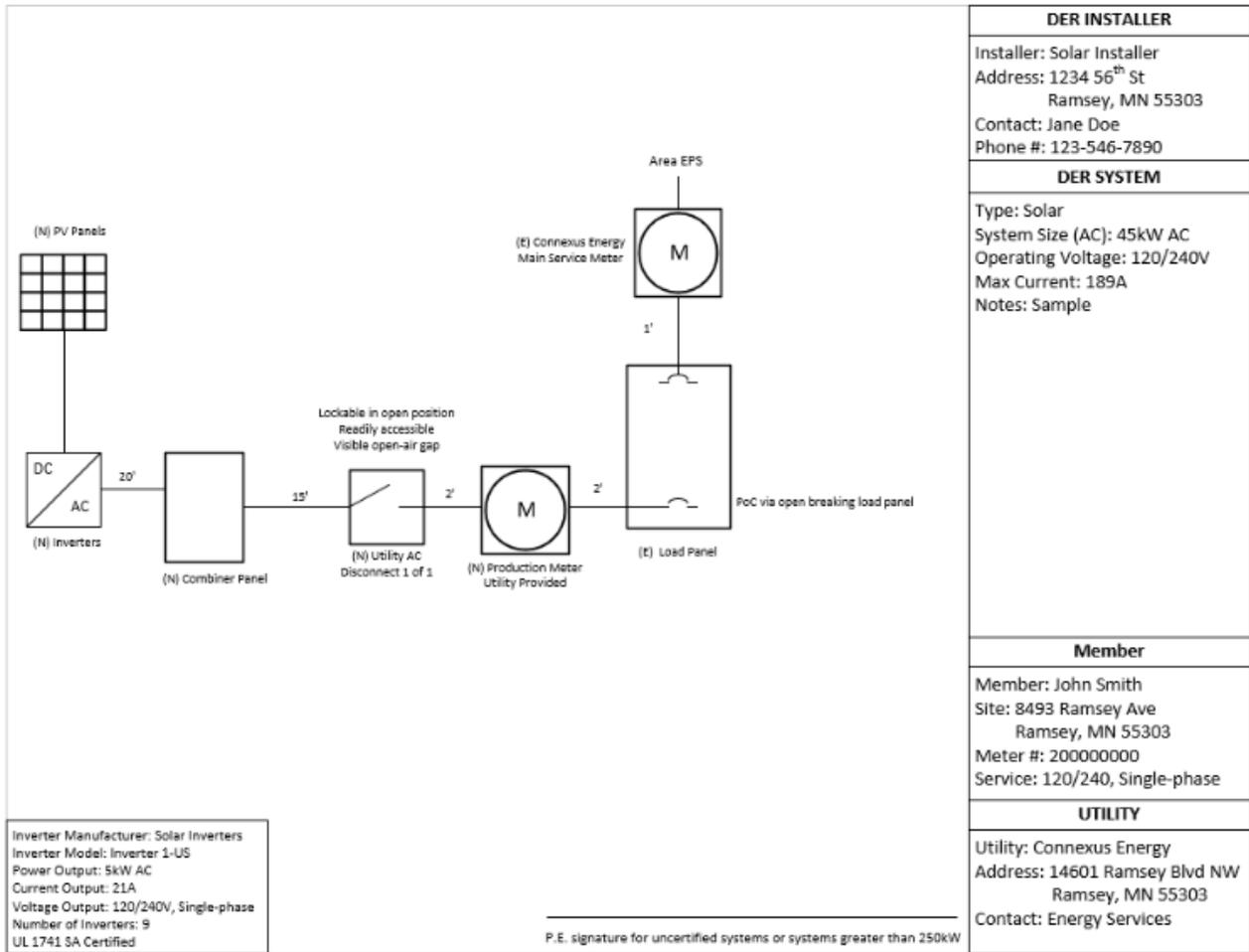
Figure 9. Example One-Line of Solar and ESS with Separate Inverters
