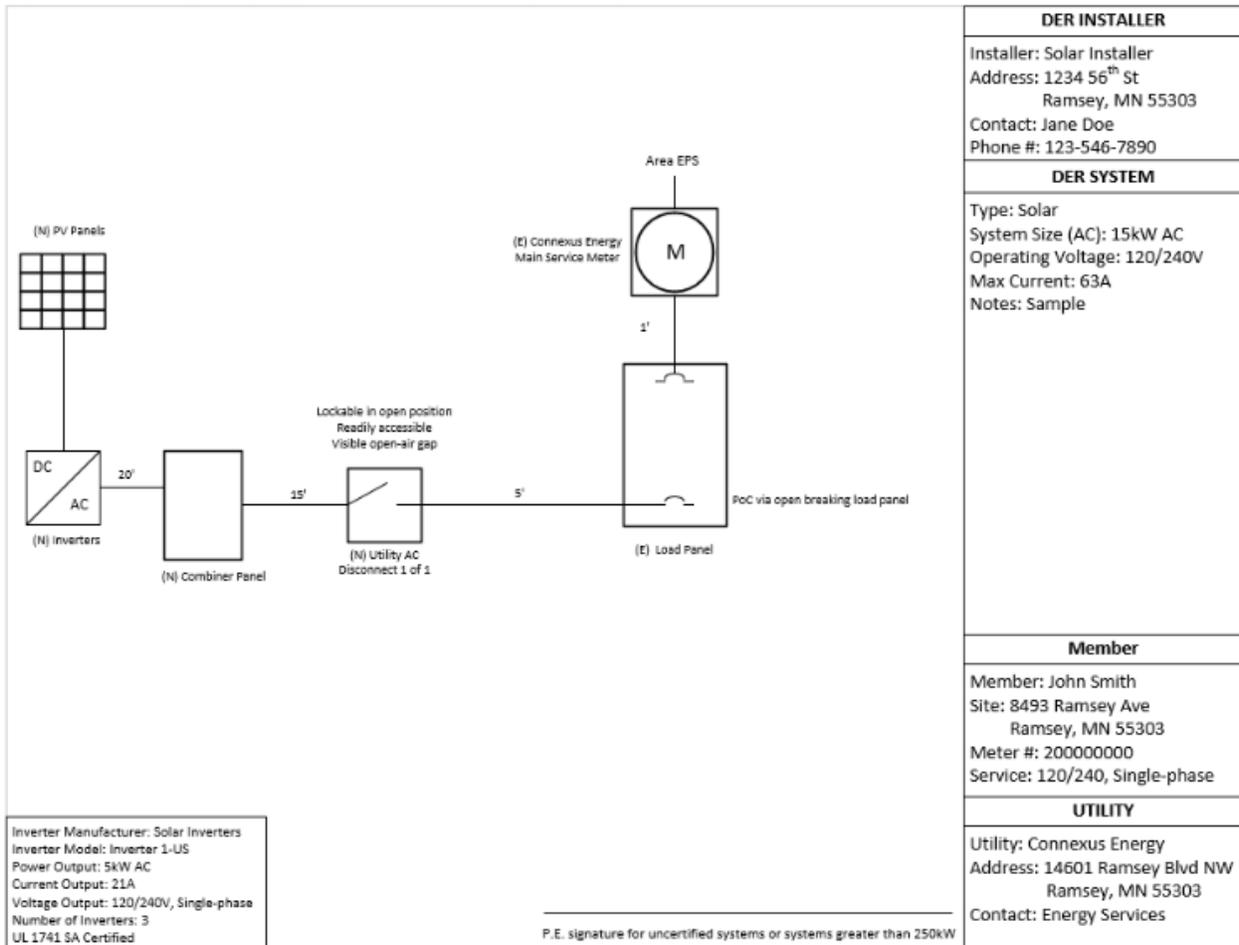
Figure 8. Example One-Line of a Solar System with a System Size Greater than 40kW
