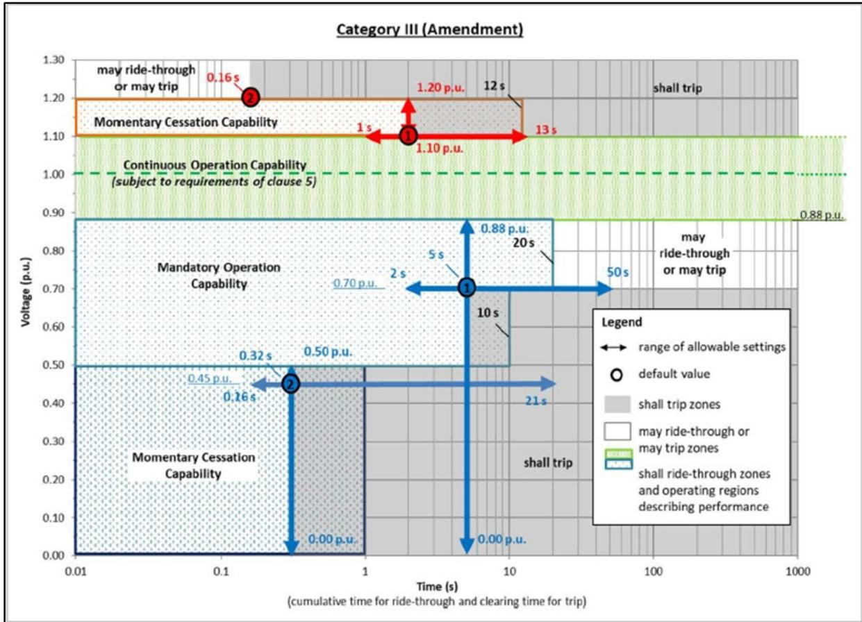
Figure 15. Category I, II and III Frequency Ride-Through for Abnormal Voltage
